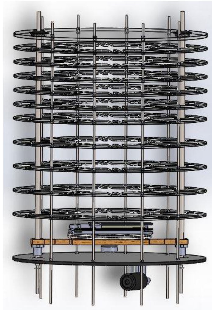
FIGURE 52: Lift System in AS/RS View
