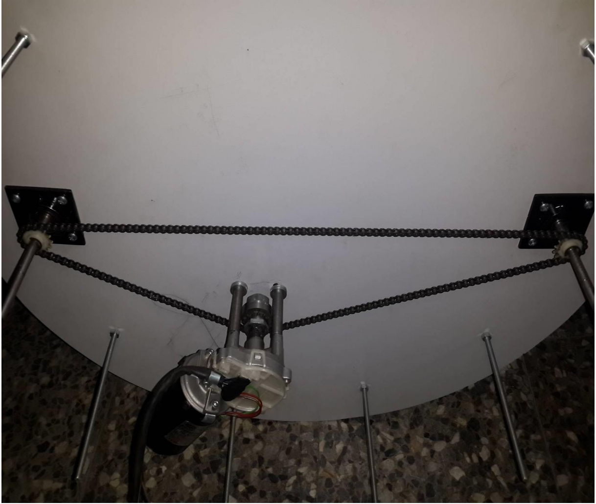
FIGURE 26: DC motor with Mils
